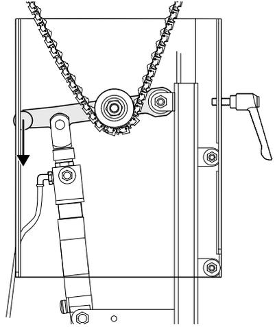
4. Move the tensioner downward until the chain is tightly secured in its position. There should be a gap of about 12.7 mm between the pneumatic-piston nut and pneumatic piston, where the piston should be visible.
