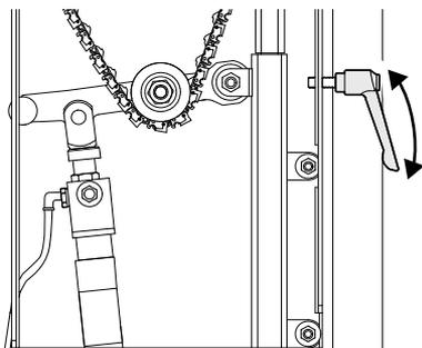
6. Gently press the chain with your hand to test the tension. The chain should not slacken.
