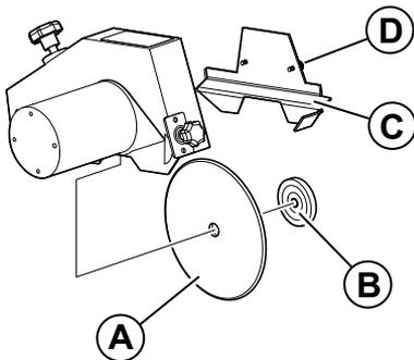
5. Remove the grinding wheel (A) from the grinding wheel axis and discard it in accordance with local, state and national laws and regulations.
