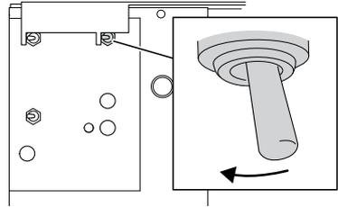
2. Set the chain pusher switch to ON to start the feeding of the chain and the movement of the grinding head. The sharpening will start after this.
