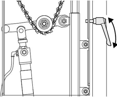
2. Lift the tensioner arm (there is a quick release function) and place the chain below the tensioner roll.
