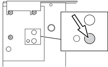
2. Set the grinding wheel switch to ON.
