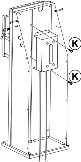
11. Next, place the machine on the stand. Fix it to the stand through the 3 holes located at the back and front of the machine with the bolts and nuts provided.
