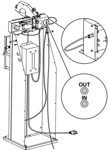
**⚠ WARNING** Attach air hoses and cables with cable clamps, to make sure no one trips over them.
