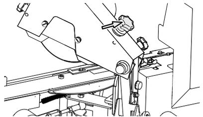
4. If required: Turn the chain pusher adjustment to make minor adjustments for the grinding length.
