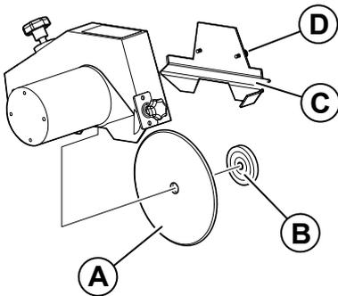
3. Remove the wheel attachment nut from the hub.
