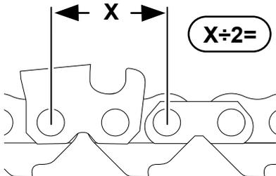
5. Loosen the chain pitch wing-nut and move it to the correct pitch position. Tighten it again.
