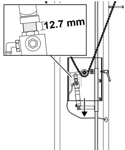
5. Tighten the locking handle to secure the chain.
