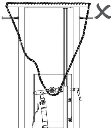
7. If the chain tension is too loose, repeat the procedure.
