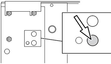
2. Press the grinding head positioning button to move the grinding head so that it is tilted in the correct start position for the next cutting link to be ground.
