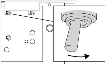
6. Lift the grinding head to its most upright position.
