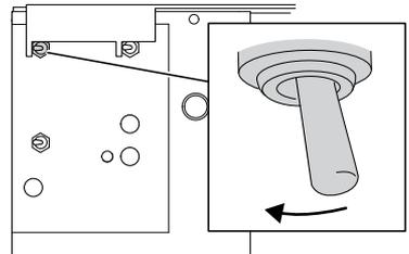
7. Visually make sure that the chain pusher stops its movement exactly above the rivet behind the cutting link, as illustrated in the image below.
