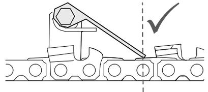
8. Set the chain pusher switch to OFF, when the grinding head is in its uppermost position and the chain lock is not engaged.
