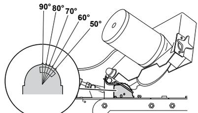
5. Change the grinding setting for the height of the depth gauges.
