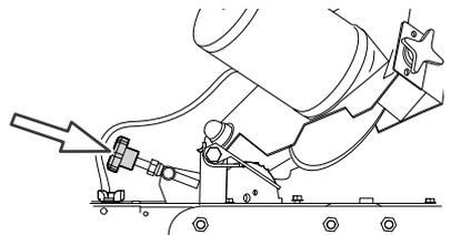
5. Set the chain pusher switch to OFF when the grinding head is in its uppermost position and the chain lock is not engaged.
