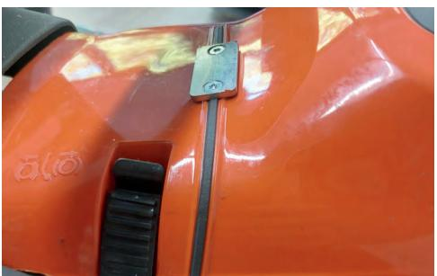
On Stihl chainsaws and older Husqvarna models we recommend to grind the marking away for example with a angle grinder.
