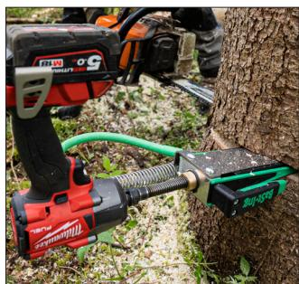
The ValFix is inserted into the tree according to the specifications in the ValFix instructions. When applying it is particularly important to ensure that the ValFix is sufficiently anchored in the tree. All nubs of the spindle wedge must be firmly seated in the wood, otherwise the ValFix may be pushed out of the cut and the tree may tip over.
