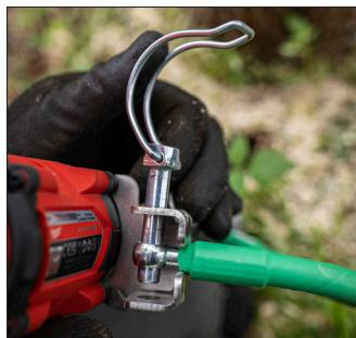
Then slide the ValLink with the linch pin (2) onto the impact wrench in the direction of the engine and attach the impact wrench attachment (3) to the impact wrench with the screws you removed.
