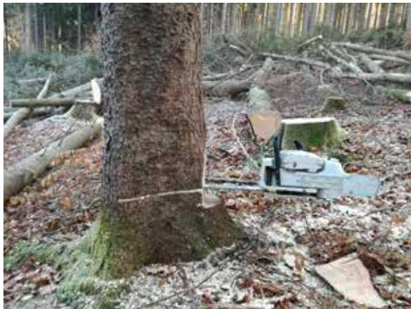
This felling cut is then extended a few millimeters, evenly upwards and downwards.
