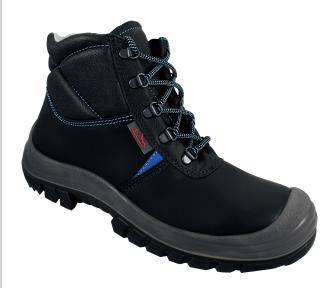
Safety shoe mid-cut form B made of full cow leather in a robust completion, special 2-layer PU outer sole with slip-resistant ActiveGrip® technology, breathable lining, light, non-magnetic and self-resetting plastic cap > 200 J load capacity, steel midsole, width 11
