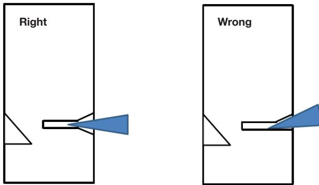
In addition, assure that the upper and lower notch-sheet (9) is equally in the tree, otherwise it can also lead to a bending of the shaft.
