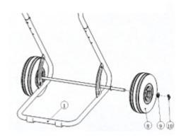
Set the axle sleeve (no. 2) on both drum sides.
