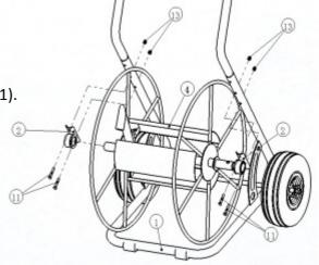
Insert the crank handle (no. 5) into the drum axle. Align the holes and affix the crank handle with the screw (M8 x 40 / no. 14), the disk Ø8 (no. 15), the spring washer Ø8 (No.16) and the nut (M8 / no. 17).
